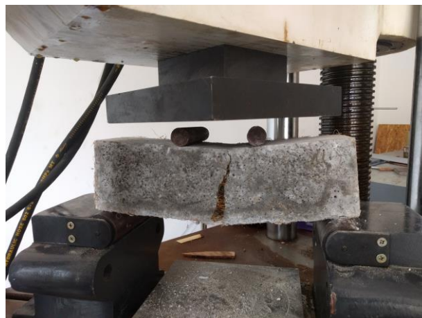
Figure 2 Flexural strength test on beam specimens
